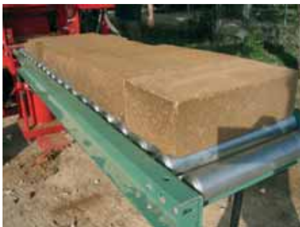
Block-making machine showing earth building blocks
